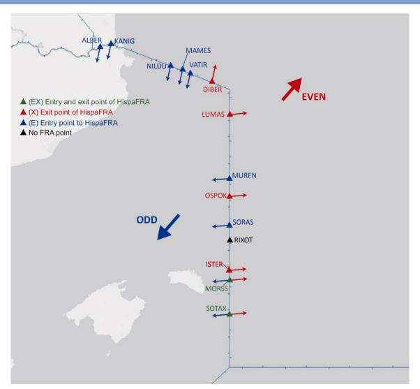
An Entry Point (E) is a published significant point on the horizontal boundary of the Free Route Airspace **from which** FRA operations are permitted, while an Exit Point (X) is a point **to which** FRA operations are permitted.
