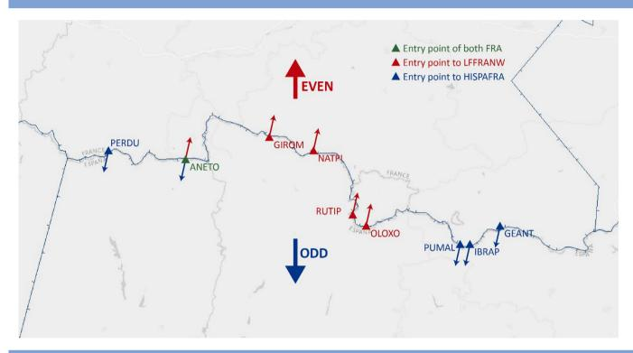
An Entry Point (E) is a published significant point on the horizontal boundary of the Free Route Airspace **from which** FRA operations are permitted, while an Exit Point (X) is a point **to which** FRA operations are permitted.
